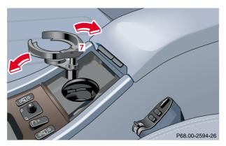
To open cup holder: Briefly press button (7). The cup holder opens automatically.
